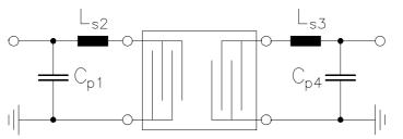
$C_{p1} = 15 \text{ pF}$   $L_{s2} = 27 \text{ nH}$   $L_{s3} = 22 \text{ nH}$   $C_{p4} = 15 \text{ pF}$
